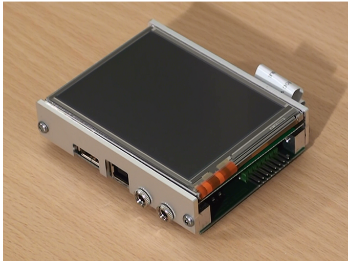
Figure 7.6: The Multimedia I/O Board with touch screen LCD display
