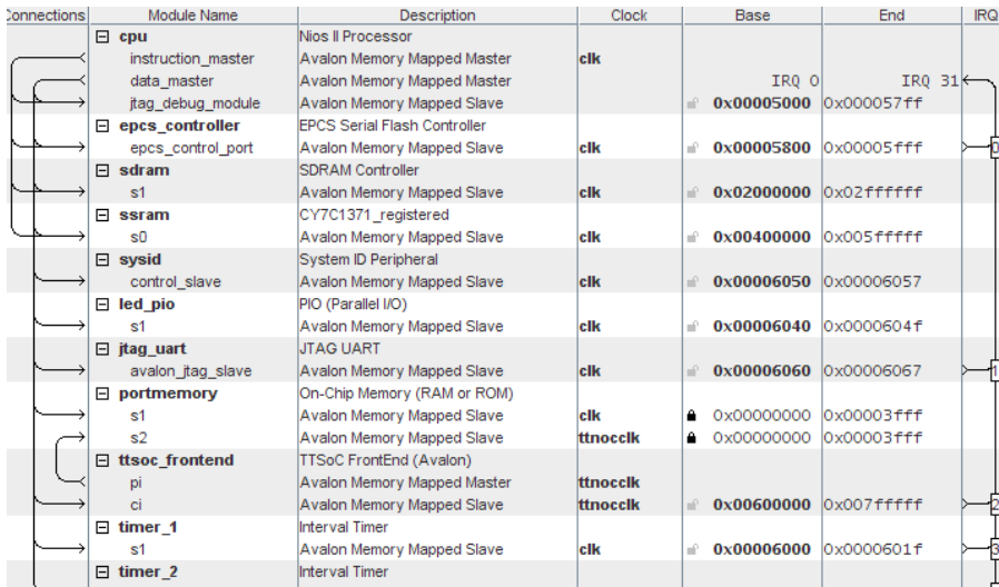
Figure 7.9: Design of the RMA and Nios II based hosts
