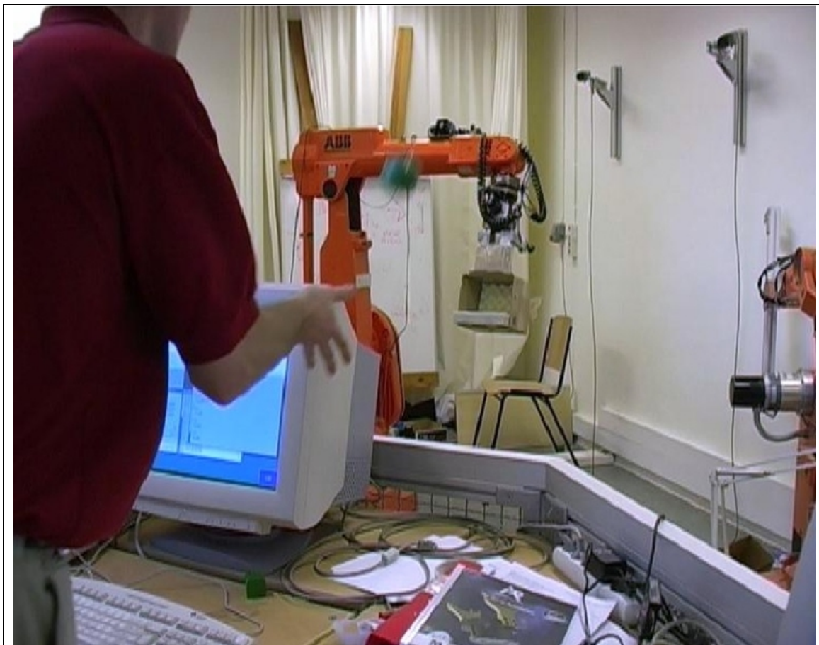
Figure 1: Experimental setup showing the two digital cameras mounted on the wall with the Irb-2000 robot ready to catch the thrown ball.
