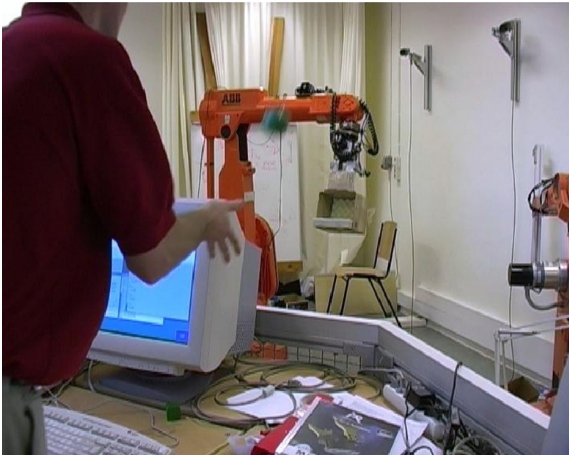
Figure 3: Experimental setup showing the two digital cameras mounted on the wall with the Irb-2000 robot ready to catch the thrown ball.
