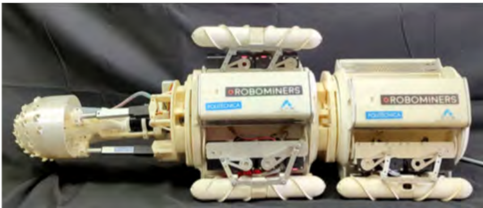
Figure 9.2: Scaled-down prototype of the miner robot composed of highly reconfigurable modular platforms, adapted from [217].
