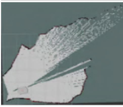
(a) Mapping results using the depth information from an RGB-D camera which has less accuracy and resolution.
