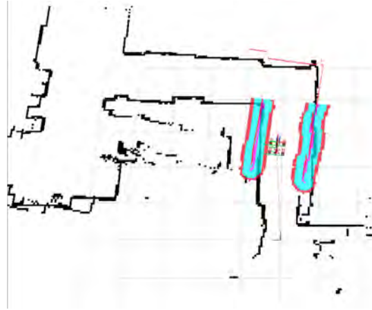
(b) Representation of the localization, map and planner output in the navigation software used for exploration. Contours of the office are delineated with distinct colors within the inflated map layer. These color differentiation affects the controller output, dynamically adjusting the vehicle's speed in response to proximity to walls and obstacles.
