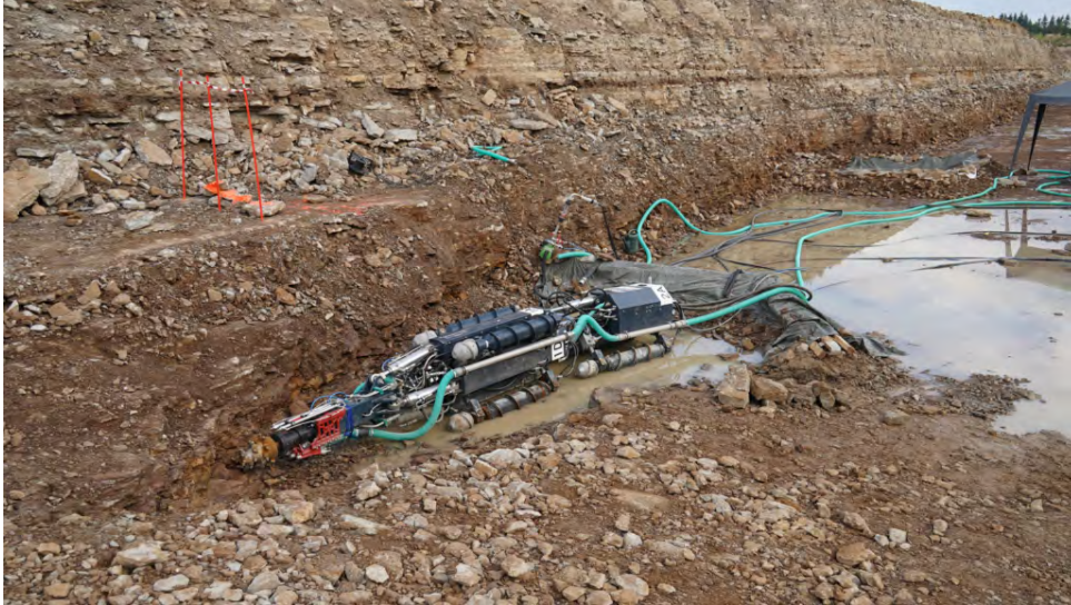
Figure 9.1: Full-scale prototype of the miner robot during field tests in the open pit, active, oil shale mine in Kunda, Estonia. Image credits: ROBOMINERS project.
