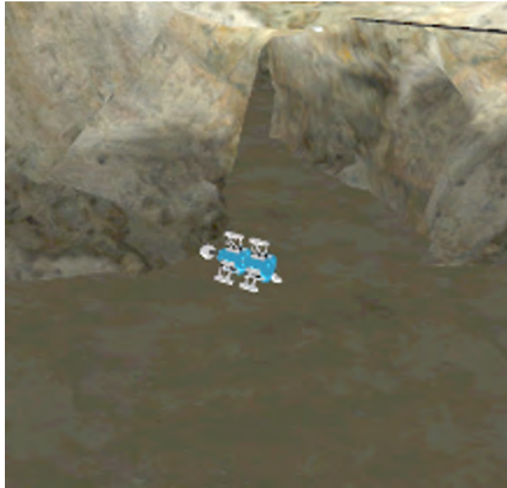
Figure 9.20: Setup after adaptation. The robotic module equipped with a cutting head has connected a spare robotic module to have more force. Now it can continue the mining task.
