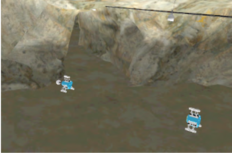
Figure 9.15: Setup for the underachieved capability scenario. On the left, a robotic module equipped with a cutting head that is used for selective mining and, on the right, a spare robotic module.
