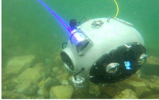
Figure 7.3: The UX-1 prototype during operation in Kaatiala Mine (Finland). Image credits: UNEXMIN project.
